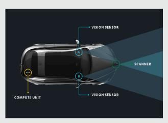
The BlincVision system consists of three different main components: a laser scanner, two vision sensors, and a compute unit. The actual placement of the components shown above may vary in a real-world scenario.
